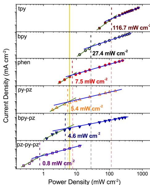
**Figure 3.** Short-circuit photocurrent density for  $\text{TiO}_2$ -A-Zn-S devices with respect to 532 nm excitation intensity ( $\text{TiO}_2$  thin-film working electrode, Pt counter electrode, with  $\text{Co}^{\text{II/III}}$  mediator in MeCN). Lines with slopes of 1 and 2 are shown in blue and green, respectively.
