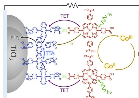
**Figure 1.** Schematic representation of the self-assembled bilayer ( $\text{TiO}_2\text{-A-Zn-S}$ ) in a DSSC with cobalt-based redox mediator. (TET = triplet energy transfer and TTA = triplet–triplet annihilation.)
